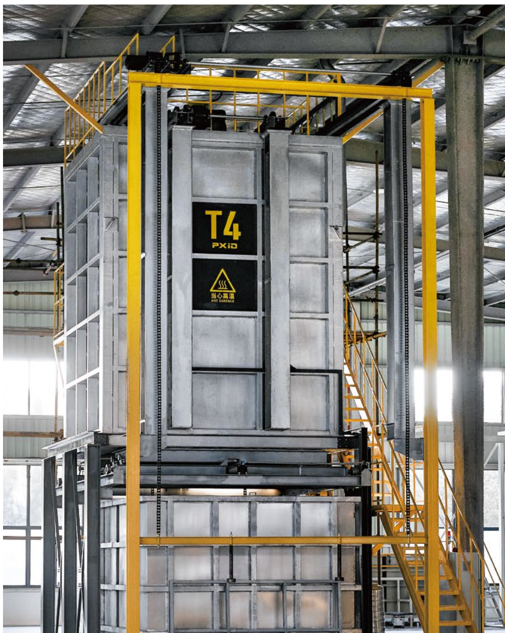
T4 T6 Frame heat treatment line
