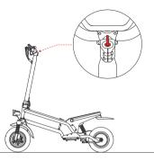
2. Power on: Turn the key clockwise to unlock and power on. And check the power indicator. If the power is too low, please charge it immediately.
