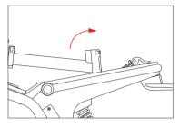
1. As shown in the figure, lift the sitting bar into an upright position.
