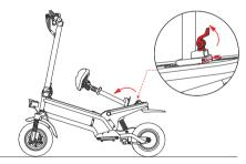
2. Open the clip as shown in the figure, push it in the direction indicated by the arrow, and then put down the column.
