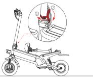
3. Rotate the buckle ① in the direction shown in the figure and open the buckle ② backward.
