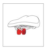
4. Unscrew the nuts on both sides as shown in the figure, and separate the lock screws from the car seat.
