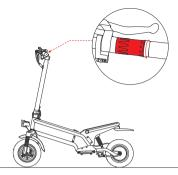
3. Start: before riding, straighten the body, adjust the sitting position, ensure it's on low speed level, turn the throttle slowly, and touch the ground with both feet; When the scooter is moving smoothly, retract your feet and place them on the pedals.
