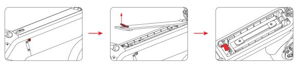
1. The battery cover on the vehicle body can be locked/opened with the special key.
