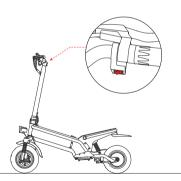
4. Speed switch: You can change speed from 1 to 3 by the speed switch .
