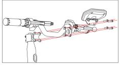
2. Place the elbow and instrument panel as shown in the figure, align the holes and tighten them with screws.
