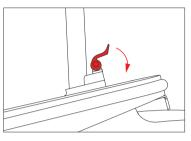
3. As shown in the figure, place the folding clasp and press it down to fix the column.
