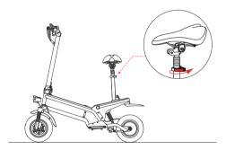
1. Rotate the buckle in the direction shown in the figure, and then rotate the car seat to the proper direction.
