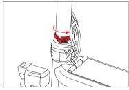
2. As shown in the figure, turn the folding wrench 3. Rotate the fixing buckle to the right as shown in the figure. Check whether the snap has been fully closed and whether the upright is firm without shaking.
