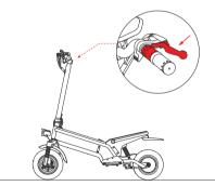
5. Decelerate/brake: release throttle to decelerate. Emergency braking requires rapid pressure on the brake handlebars.
