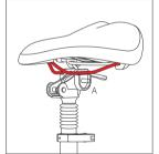
7. As shown in the figure, align the car seat with groove of compent A.
