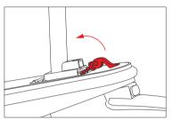
2.As shown in the figure, rotate the folding latch in the direction shown and stand in the direction of the car column to insert it into the slot
